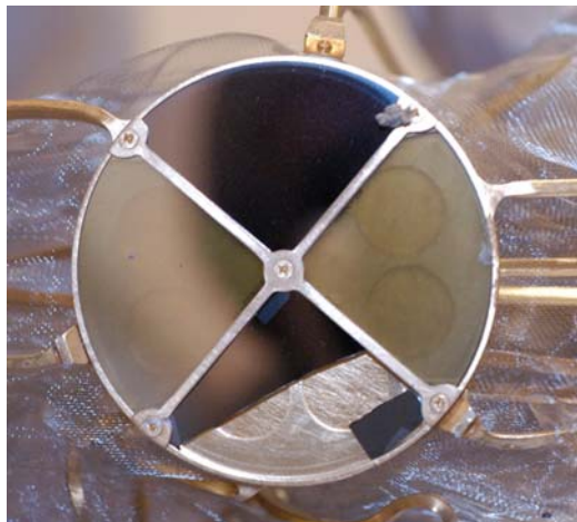
Fig. 1. Configuration of quadrants as removed from the concentrator in Utah. Additional fragments of the broken quadrant were recovered from the concentrator interior.
